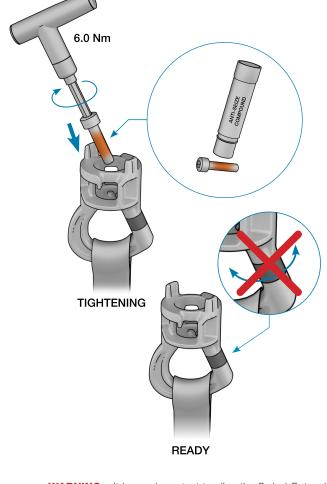
**WARNING** - It is very important to align the Swivel Gate with the internal edge of the stainless steel casting to avoid excess wear of the Auto Belay webbing
