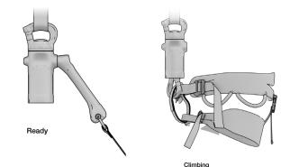
WARNING - The Ground Anchor Connector has been designed to retain the Main Body to the ground anchor point only and MUST NOT be used as a load carrying component in the fall arrest
