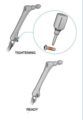
Fit the Shackle to the Ground Anchor Connector while ensuring the Shackle Bush remains in place, fit and securely tighten the Shackle Bolt.
