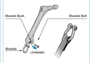
Apply Loctite 243 Threadlocker (medium strength) to the Shackle Bolt threads (ensure Loctite does not come into contact with plastic components).
