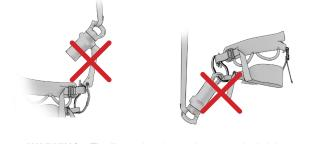
WARNING - The illustration above shows a typical sit harness. Your climbing harnesses may be of a different design. You must ensure that the Harness Connector is attached to the manufacturer's specified belay loop.
